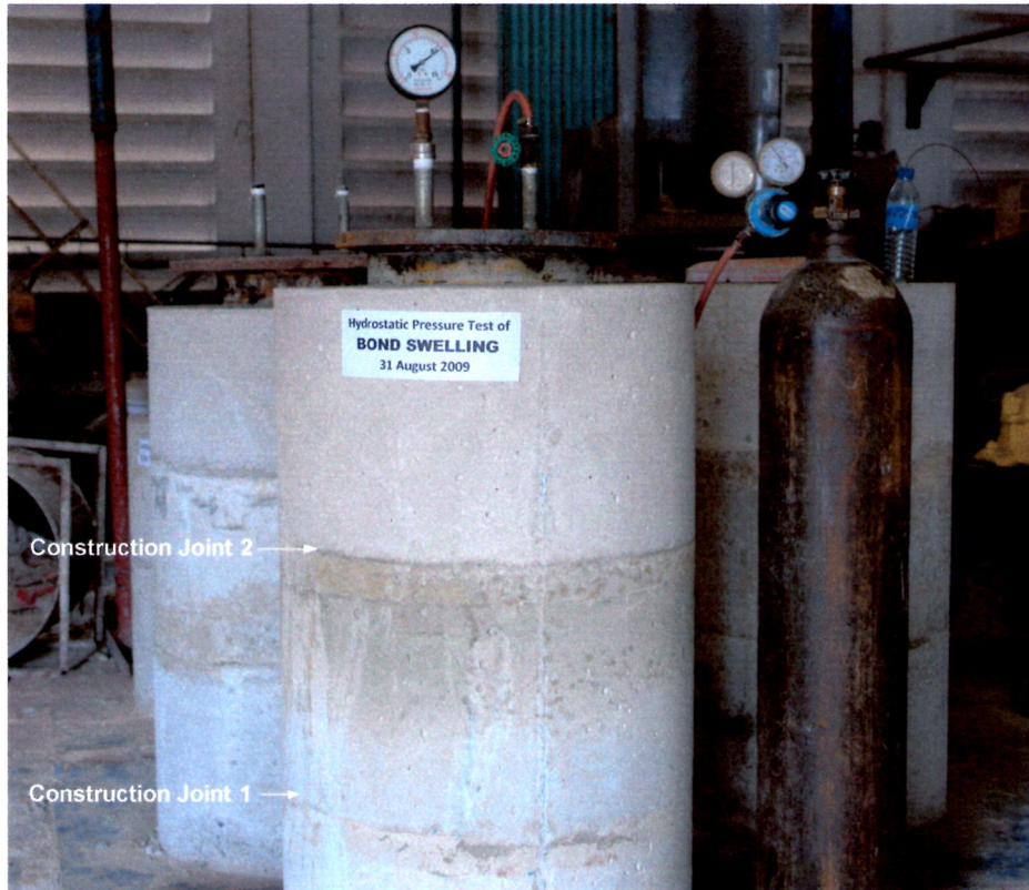
Photograph 3 – Concrete test chamber at 100 psi pressure; no leakages along the construction joints were noted.
